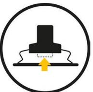
Optional pressure pad release (0.4 inches/10 mm) allows for chest rise during ventilation
