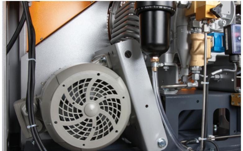
PE-HE: V-belt adjustment is likewise unnecessary in this horizontal model by use of a belt tensioning device.
