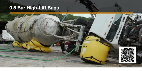
Our range of 0.5 bar pressure high-lift bags are designed primarily for the recovery of larger vehicles.
