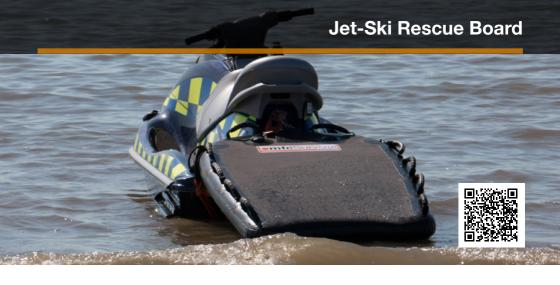
The Jet Ski Rescue Board is an inflatable board that is designed to be attached to the back of a jet ski to aid rapid response and rescue of casualties. It is attached by a towing 'D' ring and two other 'D' rings which are located at the front of the inflatable board. The board has 10 handles fitted around the top sides to make it easier for the casualty or rescue crew to hold onto the board whilst in use.
