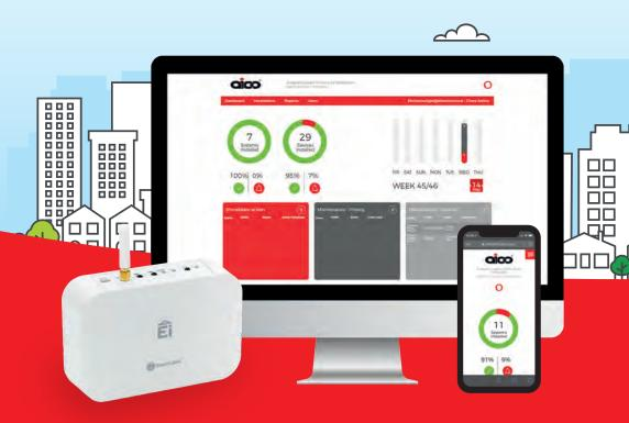
The Gateway and Cloud portal use Aico's SmartLINK technology to bring together data from all SmartLINK-enabled alarms in a property in a simple, online dashboard format – so viewing and managing them is easier and more effective.
