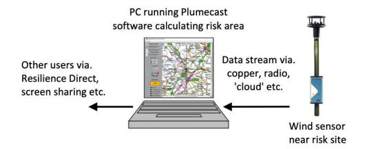
It calculates the area at risk from a release, updated every second whether an incident is occurring or not. In a real emergency it can also display the estimated present location of an airborne plume.
