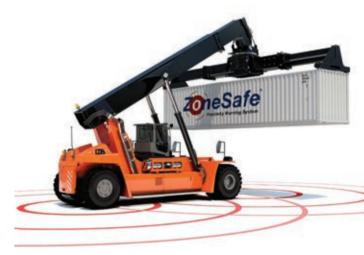
Large vehicles such as reach stackers can be fitted with multiple detection zones to cover key areas of the machine including the rear turning area, blind zones and spreaders.
