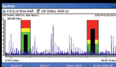
Band alarms in SPM HD spectrum
