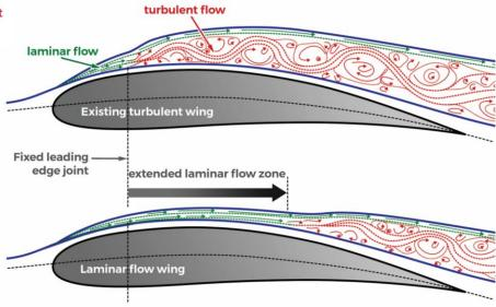
A laminar-flow-friendly FLE joint is a key technology enabler for drag reduction
