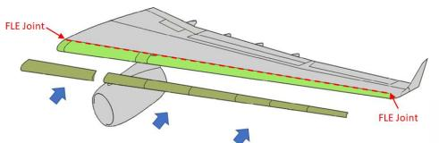
The Fixed Leading Edge (FLE) joint (as a flow disturbance) is a significant threat to maintaining laminar flow across the rest of the wing chord
