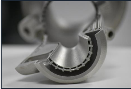
Combustion Chambers 291 mm, Ø147 mm
