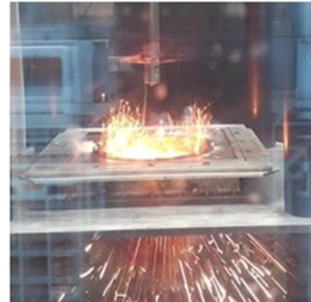
Lightning strike testing of composite baseplates
