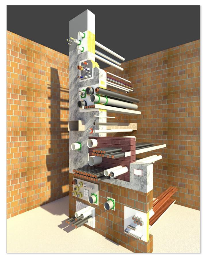
Mixed penetration sealing system made of mineral-fibre boards and ablative coating. Fire resistance - up to El 240 min.
