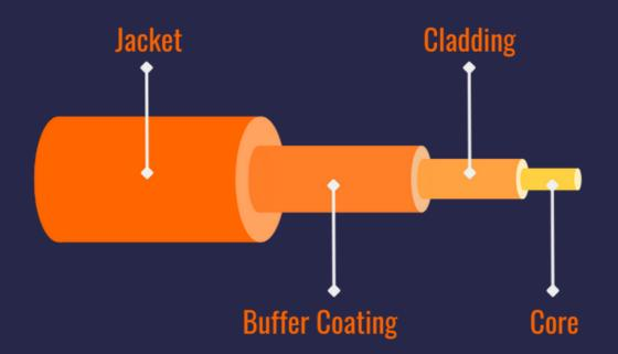
The core of fibre optic cables is measured in microns ( $\mu$ m). The core size of multimode fibre cables is 50 $\mu$ m and 62.5 $\mu$ m, while single-mode fibre cables are measured in 8-9 $\mu$ m.
