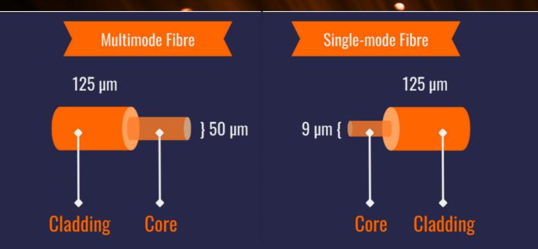
Fibre optics carry different frequencies of light or wavelengths. When measuring Fibre optic wavelengths we use nanometers, with MMF wavelengths measuring 850nm and 1300nm, and SMF wavelengths measuring 1310nm and 1550nm.
