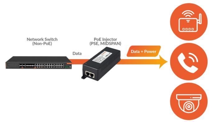
The key difference between Endspans and Midspans is the location where the power is injected into the Ethernet cable. Endspans inject power from within the network switch, while Midspans inject power from an external device. This can affect the overall network architecture and the number of devices that can be powered using PoE.
