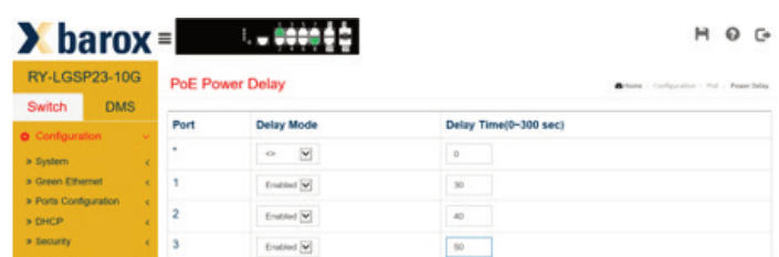
Fig.4 barox RY-LGSP23-10G PoE Power Delay
