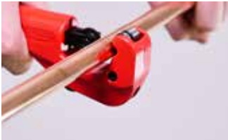
1. Cut the tube to length
