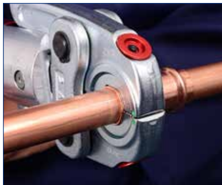
5. Complete joint with the press tool
