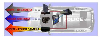
The Application analyses continuously the car plates, checks toward downloaded Authority registers (up-to 3 register). When Hit takes in place it is notified by Voice and Colour-signal. Colour-signal signifies the severity of Hit.
