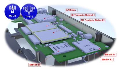
There is optionally platforms for 1 or 2 Modems for Client applications and in addition 1 modem for IoT-interface. Modem-types are selective according to the Clients options.
