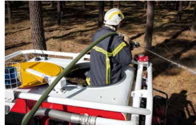
Fighting fires from the roof hatch, available ex factory.
