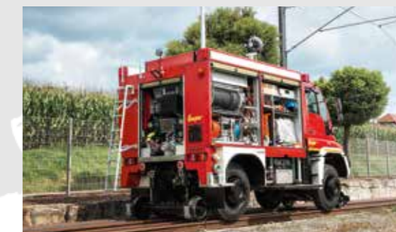
Emergency response on road and rail in Istanbul, Turkey. The versatile road-rail Unimog with hydraulically elevated rail guidance system can reach the site of an incident by road at speeds of up to 90 km/h and then switch to rail drive, for example in tunnel rescue operations.
