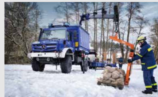
Emergency response vehicle with rear-mounted crane and boat trailer. The rescue workers at the Technisches Hilfswerk rely on vehicles with extreme off-road capabilities. Unimog U 5023 protect a region of Bavaria which is at particularly high risk from flooding.
