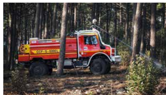
Fighting forest fires in the south-west of France. Every year 687000 hectares of pine forests are threatened by forest fires. To tackle the flames, the Unimog has 5500 litres of water on board, a self-protection system and a round roof hatch to enable it to fight forest fires on the front line.
