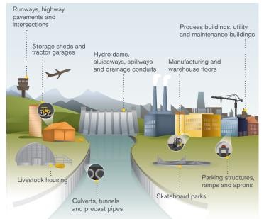
Areas where abrasion and erosion resistant concrete is needed.
