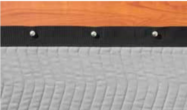
Securely hang Palmer StudStrip® elevator pads from cab studs without grommets or additional hardware. StudStrip® pads are made from black heavy-duty slotted webbing sewn to the top of vinyl or canvas pads. Palmer StudStrip® eliminates time consuming grommet measurements with durable 5/8" stud slits spaced 1" apart. **Patent pending.**
