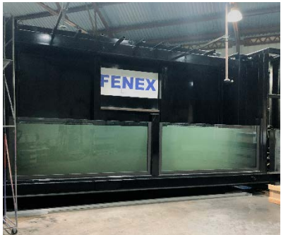
4x8' Sections Holding 4' of Water
