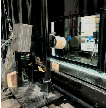
Impact Test on 4' x 6' Flood Window
