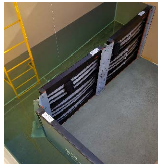
Corner Sections Tested Under Load
