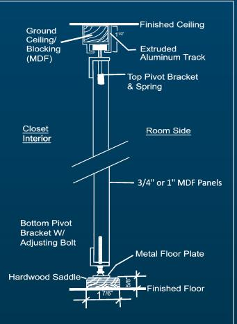
**Side Elevation.** The panels are available primed or pre-finished MDF, not particleboard. Installations can be done with or without the hardwood saddle, and door panel heights and reveals are calculated accordingly. Our doors are much simpler to install than our competitors and eliminates extra components like door stops, springs notched into panels, vinyl bumpers, snubbers and magnetic catches.
