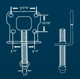
Bottom Pivot allows the Paniflex™ system to be adjustable for openings that are not square by a 1/2 inch taller or shorter.
