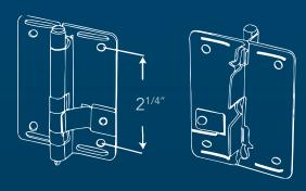
Patented TruClose™ Hinge cam tab and oblong hinge barrel shape create a self-closing effect. This helps the door close smoothly and once closed, keeps it there. This system replaced the piano hinge we used back in the 1950's and 60's.
