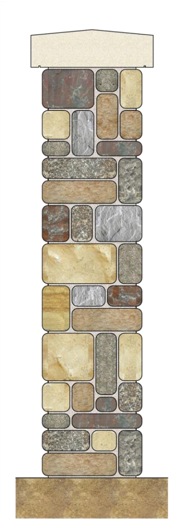
Mass rubble wall
