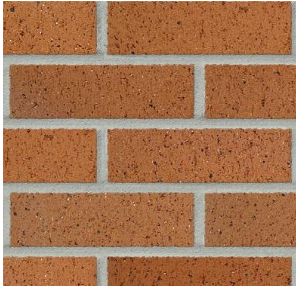
ONE SQUARE FOOT MODULAR BRICK, RUNNING BOND
