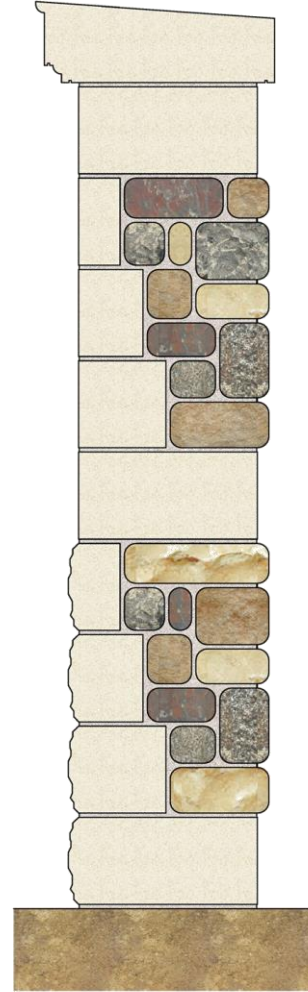
Ashlar wall w/ rubble backing
