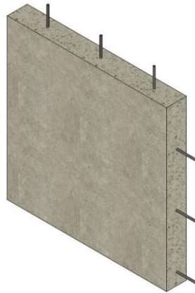
A16 Concrete, cast-in-place
