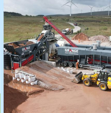
Cement / PFA material wet batch plants designed for high output production and the continuous production of concrete.
