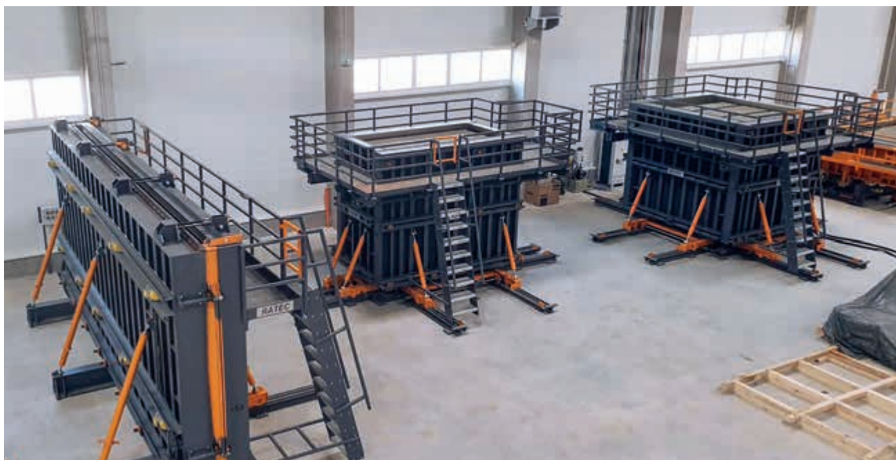
View of the factory, here with 2 modular moulds, a vertical roof mould (top left) and variable basement mould (bottom)
