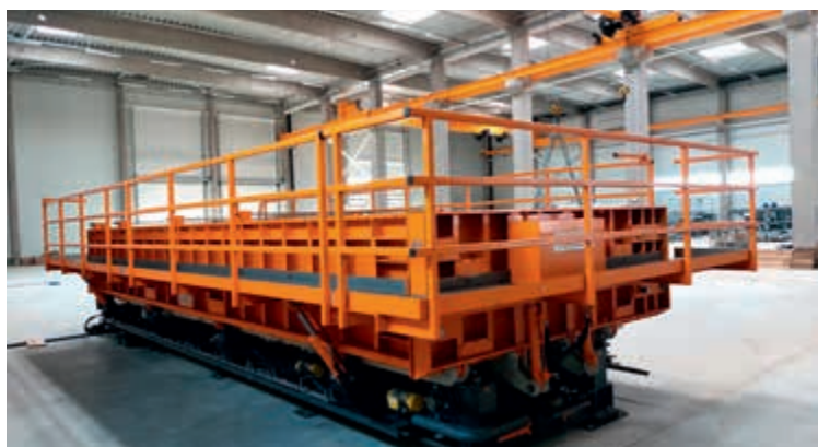
View of the factory, here with 2 modular moulds, a vertical roof mould (top left) and variable basement mould (bottom)
