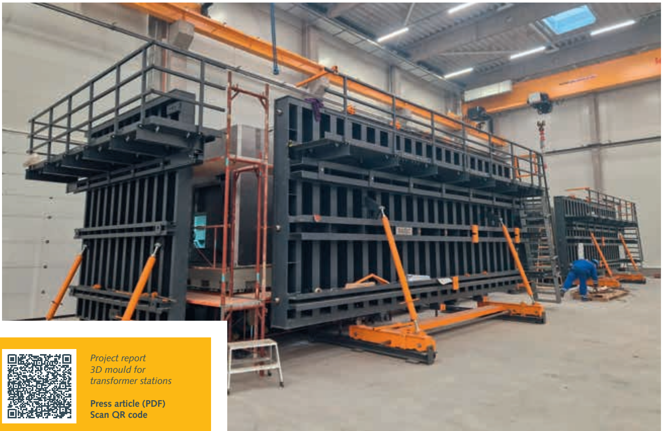
Adjustable mould for elements from 3 m to 8 m in length
