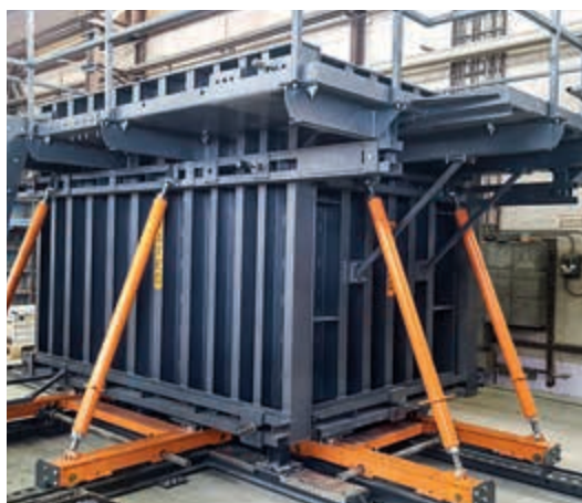
Example: Mould for the production of transformer stations measuring 2.4 x 2.1 x 2.3 m and 2.9 x 2.1 x 2.3 m
