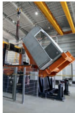
Left: 3D mould kit for multi-storey modular construction with complex details
