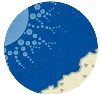
Crystals produced by the hydration reaction grow away from each cement particle during curing.
