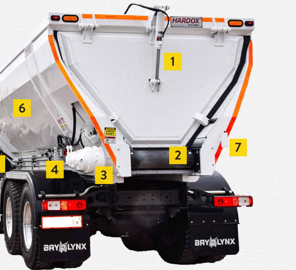
**1. Hydraulic Tailgate** - Hydraulic cylinder for partial tailgate opening and controlled discharge.
