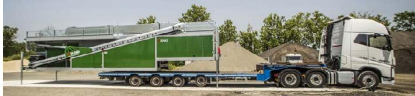
A240 is a high-capacity truly mobile and fully autonomous plant that can do a wide range of mixes and doesn't require cranes for installation. It can easily be transported on a flat bed trailer without any special permissions. It is a unique solution with a Twin Shaft mixer that revolutionises the volumetric plant capabilities. In addition, negative weighing principle for cement and aggregates provides highest accuracy.
