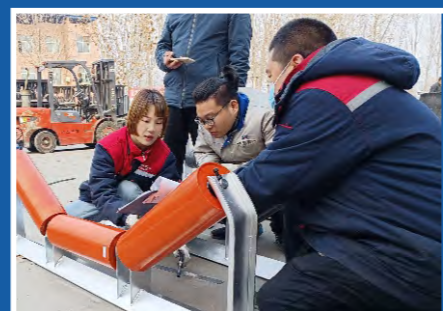
Idler Dimensions Inspection
