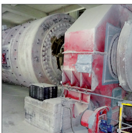
Portlandzementwerk Wittekind with a CJC® Fine Filter installed at the main gearbox of the cement mill ZM I
