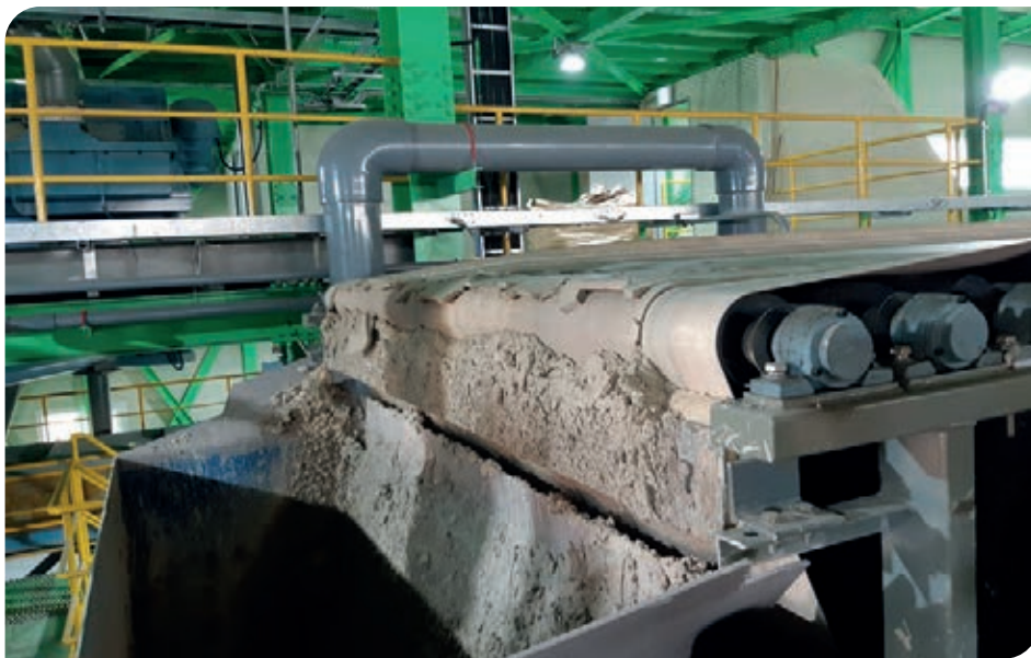
Figure 6: Filter cake (cleaned bypass dust) at the outlet of the vacuum belt filter.
