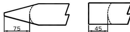
Flat type chisel worn more than 45mm or moil type and wedge, universal type chisels worn back more than 75mm of working end classed as reasonable life. Warranty claims rejected.
