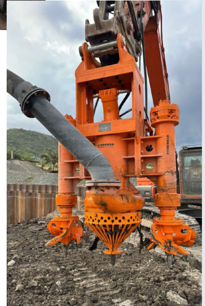
200THY55-6P + 2 Expro-7.5 Fit for Komatsu PC300 for Sand Extraction. (Philippines)
