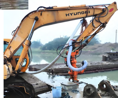
200THY75-6P Coupled on Excavator 36t HX Hyundai. (Australia)
