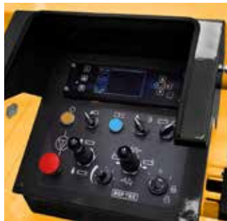
Above: The main control panel is complimented by a radio-remote control unit.
