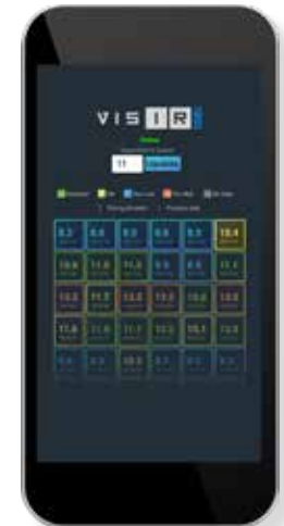
Above: VISIR-ROS software reports on the amount of chippings that have been distributed per square metre.
