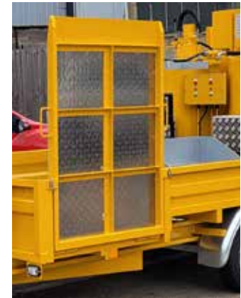
Above: Ramp fitted to nearside for loading equipment.
