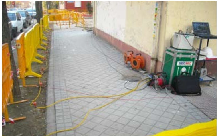
Figure 3: Implantation and performance of diagnostic 3D E.R.T. tests.
