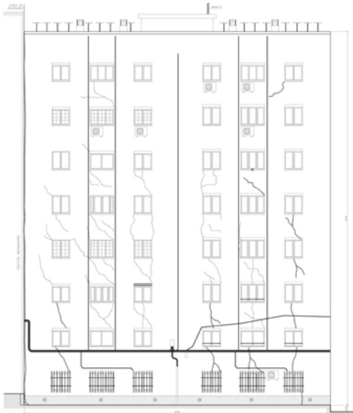
Figure 3: Implantation and performance of diagnostic 3D E.R.T. tests.
