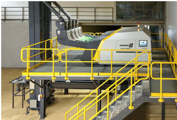
Caption: UniSort Finealyse®+ for sorting fine-grain bulk material like plastic mixes, copper scrap and heavy metal and non-ferrous metal concentrates. Photo: STEINERT
