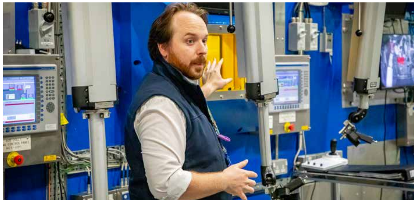
A pair of mechanically coupled remote manipulators is shown to the right of the operator as he stands in front of the shield wall of a Hot Cell in the MRF. The yellow shape is a pane of glass with lead for additional shielding. This wall and window are very thick.
