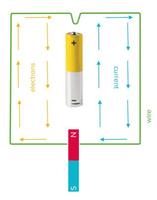
The current flows from the positive terminal (with the bump), through the wires down to the magnets, then back into the negative terminal. Due to convention, electrons move in the opposite direction to current flow.
