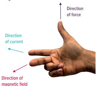
When you add the right hand rule on to the diagram, the current is flowing down the wires on the outsides (blue arrow on hands). The magnetic field is going away from the magnet (i.e. left on the left side and right on the right side, red arrows on hands) and the force is therefore the thumb (purple arrow on hands, running into the page on the left and out of the page on the right). Therefore, if viewed from the top, this setup would spin clockwise.
