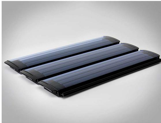
The Mast(eR) profile is the standard 60 mm profile in polycarbonate and in white and grey PVC. Height 14 mm and an uplift of 8.14 Kg/m<sup>2</sup>, Perfect geometry to replace any other profile. Because of its compact sz, this slat is applicable in every situation, both in new buildings and renovations. It can be mounted above ground or under water.
