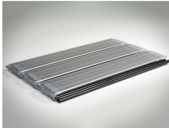
The Clean(eR) Profile is also 60 mm wide and has an extra dark chamber to reduce the formation of algae in the hook connections. The Clean(eR) Profile in Polycarbonate Solar is available in different colours. The Clean(eR) Profile is 15 mm high and therefore has a larger total roller diameter. Due to the extra closed space, the upward force is also higher: 9.6 Kg/m<sup>2</sup>.
