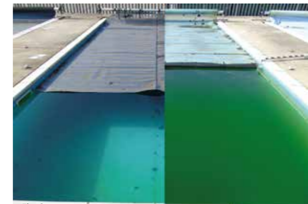
Fig. 3 The above composite image (Fig. 3) shows pools covered with EnergyGuard™ Selective Transmission (L) and a transparent cover (R) over the winter period.
