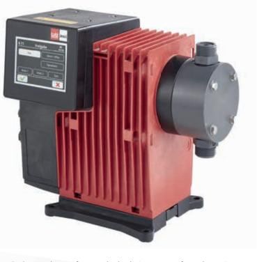
For low supply rates, for example, the dosing pump performs the suction stroke at the maximum speed and adjusts the speed of the pressure stroke to match the desired supply rate. This produces an almost constant supply stream, which enables low-pulsation, low stress dosing.
