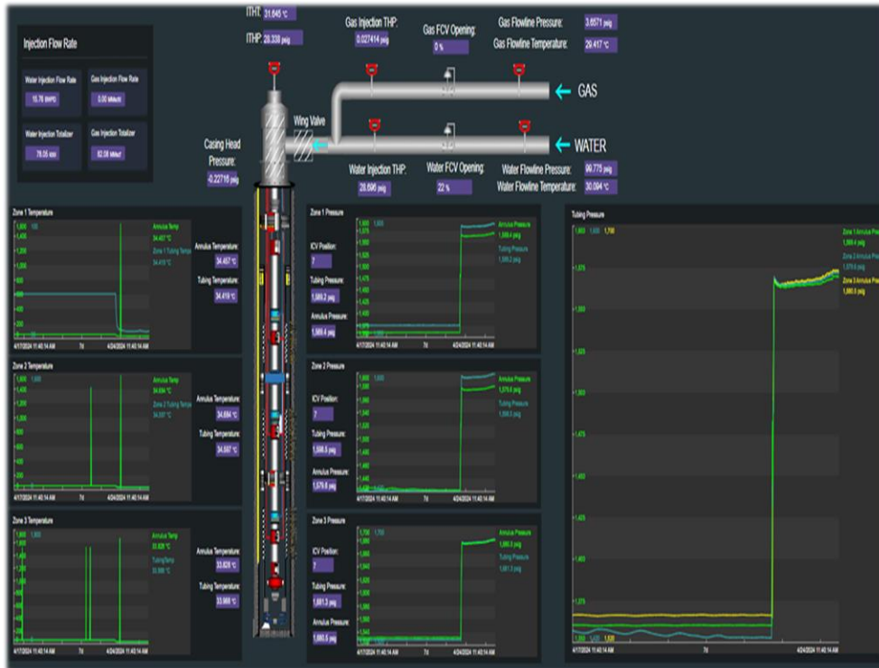
(1) Injector Wells Key Parameters Monitoring
