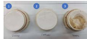
Fine Filter slope test result (3) with traces of garnet
