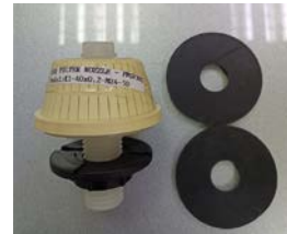
Mushroom cap installed with Loctite
