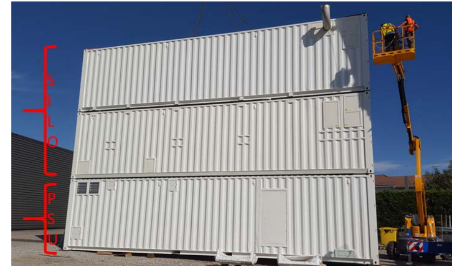
Bulk pneumatic delivery: new double container horizontal bulk silo and dissolution unit general outside appearance
