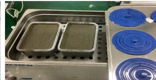
Preliminary curing and molding of the cement slurry ↓
