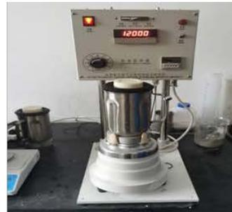
Mixing and stirring of the cement slurry →
