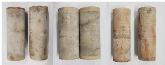
Corrosion tests of cement with supercritical CO<sub>2</sub>
