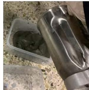
Vibration of the cement slurry for 15 minutes →
