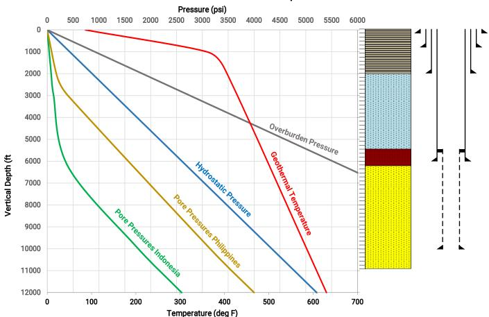
Sub hydrostatic pore pressures.
