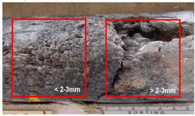
Smaller fractures < 2- 3 mm cause fluid losses when drilled overbalanced.
