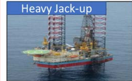
Self-Propelled Jack Up Barge or Cantilevered Lift-Boat equipped with Workover Unit / P&A spread
