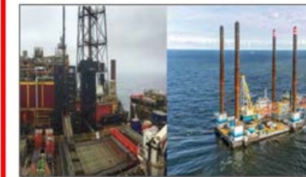
Self-Propelled Jack Up Barge or Cantilevered Lift-Boat equipped with Workover Unit / P&A spread
