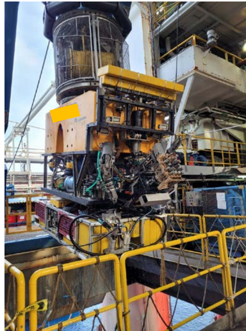
ROV with Injection Skid
