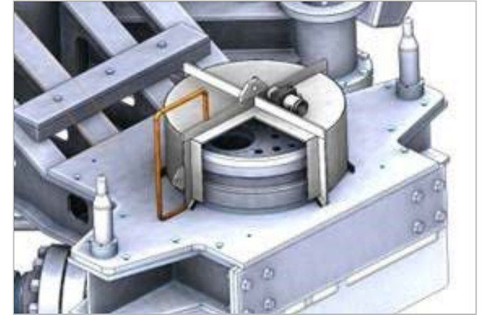
Figure 1: Shroud Design for Negative Buoyancy Agent (courtesy of TMT)
