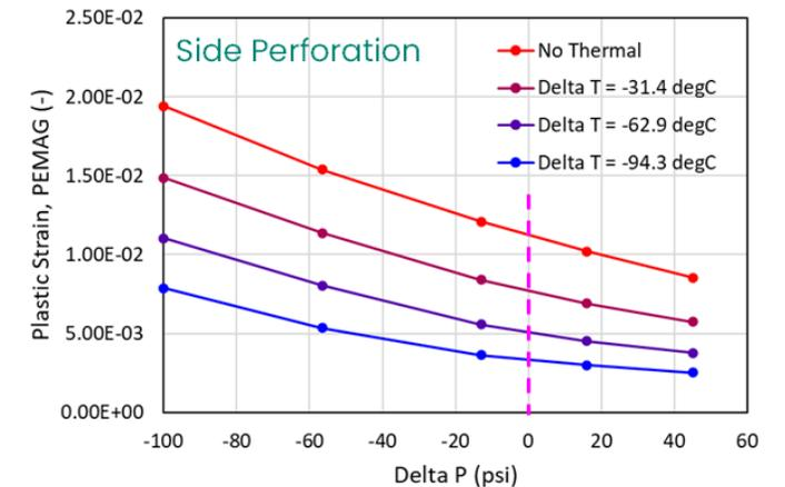
Thermal effect on the plastic strain for different perforation orientation during injection (Higher cooling effect reduces plastic strain as compared to no thermal effect)
