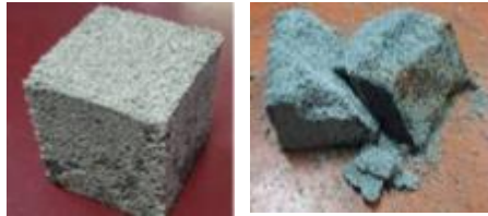
Cured resin sample SandTrap 225/350
